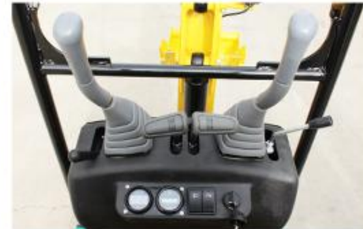
Operating rod Hydraulic pilot operation
