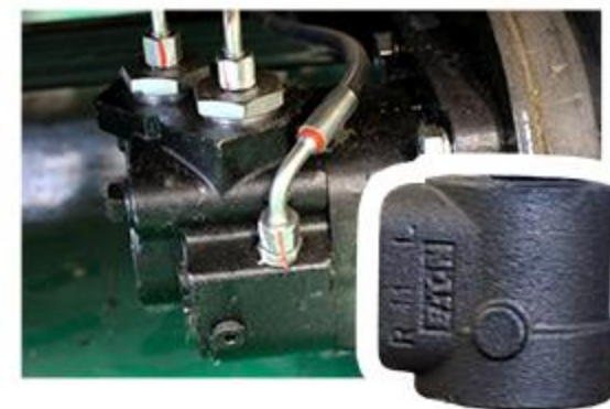
Walking motor American Eaton motor, with a sealing ring inside
