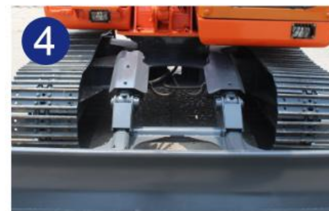
4 Bullboard using a casting process to connect the central support, strong and durable
