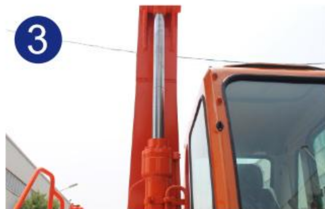
3 Cylinder Engineering specific, sealing ring for American Pike, with buffer device
