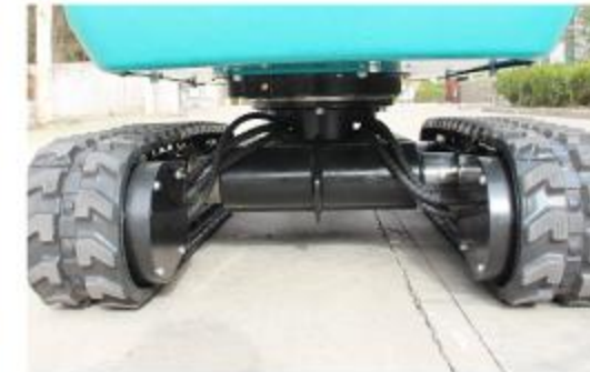
Retractable track Convenient for narrow space operation
